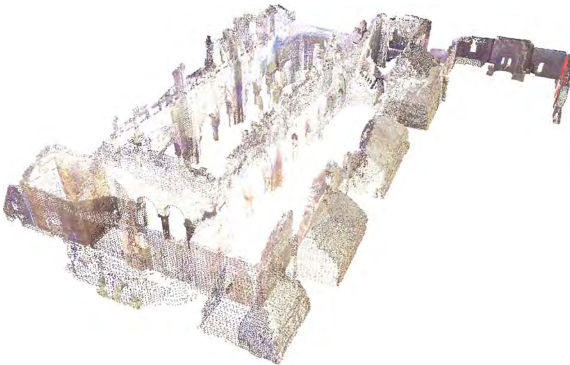
Fig. 13: Resafa, Basilica A, filtered TLS point-cloud, view from southwest (D. Kowoll/A. Sternberg, 2007).
